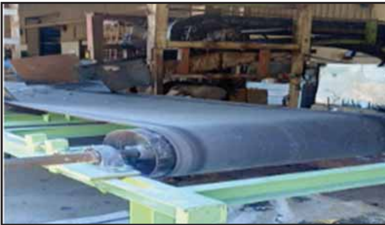
▲ Installation of Scrap handling conveyor at Stamping Division ▼
