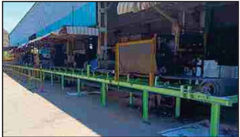
▲ Installation of Scrap handling conveyor at Stamping Division ▼
